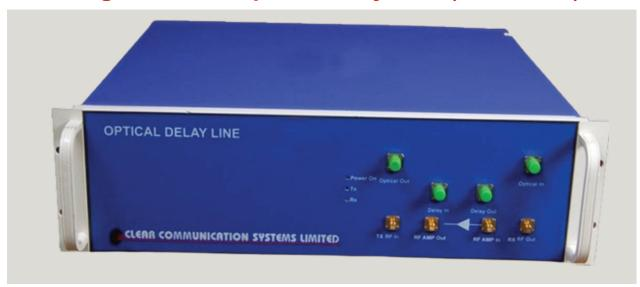
Programmable Optical Delay Line for RF and Microwave applications uses low loss optical fiber with specific delay, based on the length of the optical fiber selected. The time delay is achieved by selectively routing the optical signal through a set of fiber segments with required length. The 19" rack mountable module provides digitally variable time delay from 20ns to 1500ns with a step size of 5 ns.
